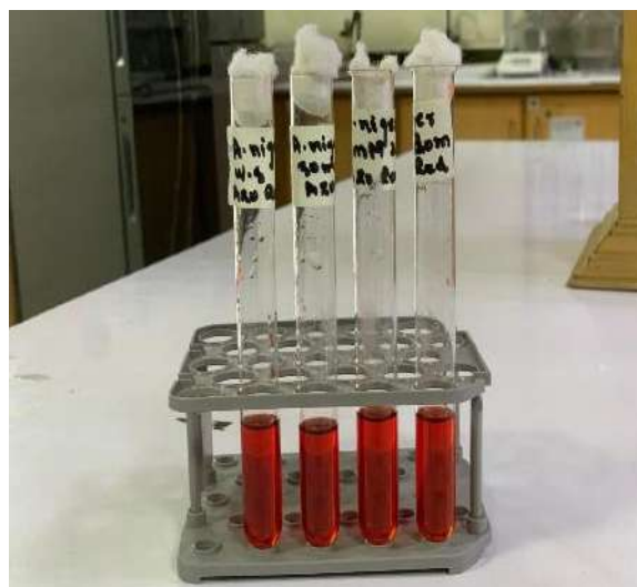
Figure 18: After incubation for 72 hours of Congo red dye for A. niger strains. Baseline absorbance of Congo Red dye at 497 nm before incubation with wild and mutated Aspergillus niger strains,
